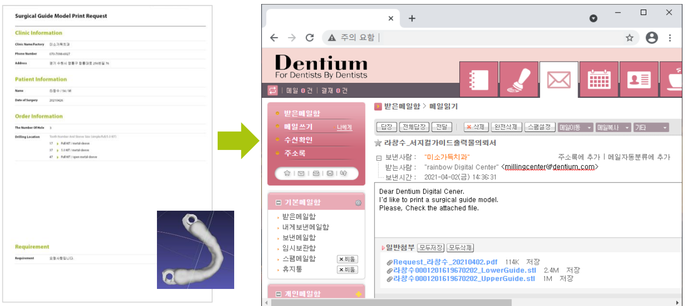
Transmit Surgical guide model output request in PDF file and STL file to the milling center
