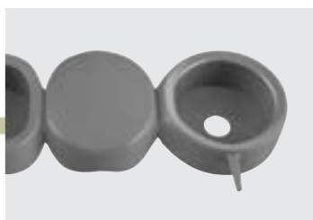
Metal framework after removal of "Lip"
